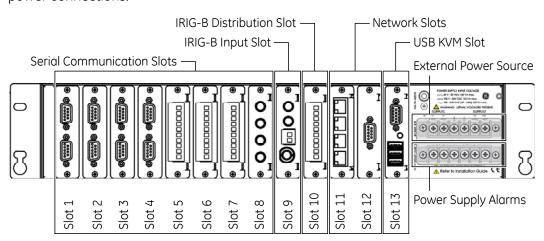
The D400 contains 13 I/O adapter card slots for the communication cards. The communication cards are powered from the backplane of the D400. The types of communication cards included in your D400 depend on what was ordered for your substation application.
